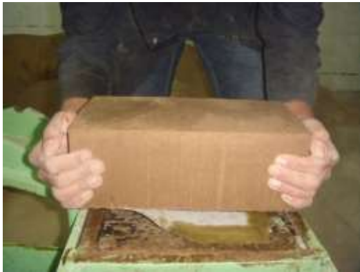
Figure.3 Ready brick for curing
