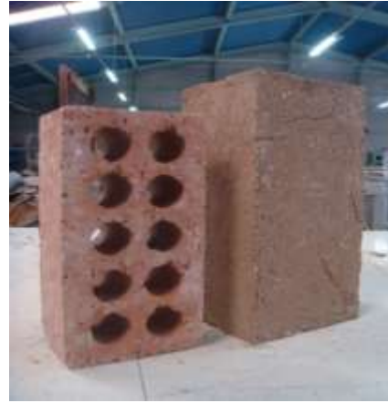
Figure.4 Laboratory-produced unfired brick compared with fired brick
