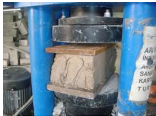
Figure.5 Appearance of failure after compressive test
